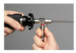
3. Attach the light to the scope by pressing its quick connect/release at the top of the light.
