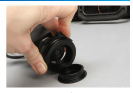
1. Remove the lens cap of the camera c-mount coupler by rotating the coupler's quick connect/release.
